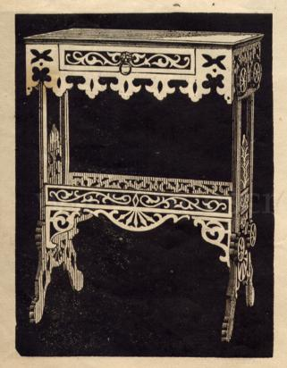
Sides are sections and should be sawed from 1/2 inch material. Can be made with a hand saw.
