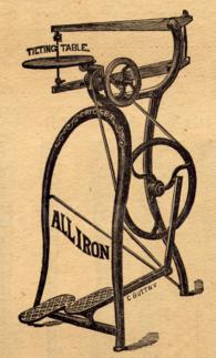
To meet the demand for a cheap and good Foot Power Saw, we have made an all Iron Machine, which we offer for \$3.00. The finish is the same as our Lester and Rodgers Saws. Weight of Saw 17 pounds. Weight when boxed, 35 pounds. Just as good as any Jigger in the market. Price, \$3.00.
