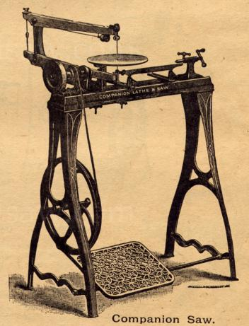
The Lathe Bed is 24 inches long, fifteen inches between centres, and five inches swing. The Scroll Saw can be taken off by loosening one bolt. Both the Lathe and Scroll Saw have all the improvements, all the tools, patterns, and accompaniments, which go with our other machines. The quality and price of this Companion Saw will ensure it a very large sale,
